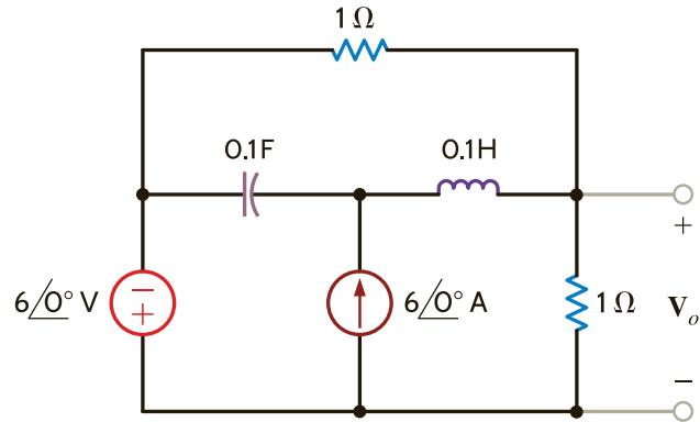
Calculate the average power absorbed by each of the circuit elements.
