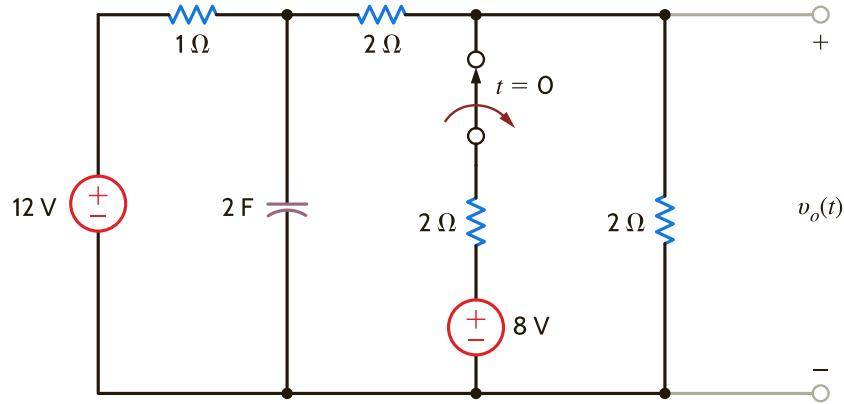
Assume that the circuit reaches steady state after a duration equal to five times the time constant. **Calculate the exact time at which the circuit reaches steady state.**
