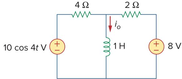
a) Find  $i_{o1}$  due to  $8\text{ V}$  voltage source.  $i_{o1} = \underline{\hspace{2cm}}$
