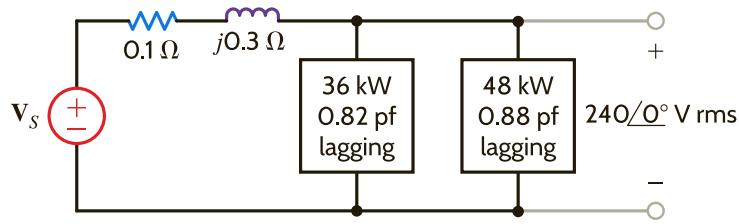
Find the total complex power at the load  $\mathbf{S}_L$ , the total current  $\mathbf{I}_L$ , and the equivalent load impedance  $\mathbf{Z}_L$ .
